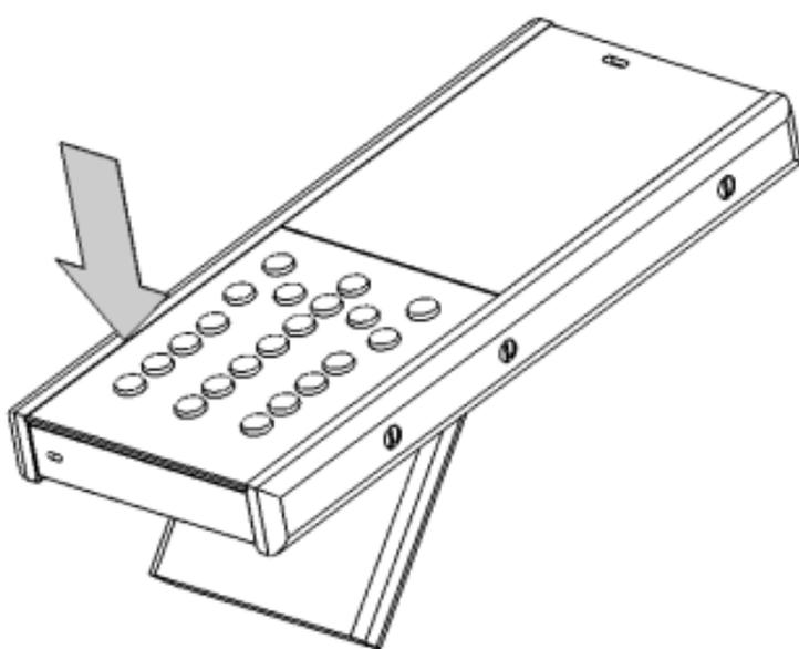
Insert the SIM card. Make sure the golden contact area is facing downwards and is oriented as shown. Replace the battery as shown.
