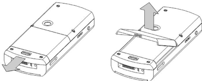
Remove battery by lifting. Pull up the locking clip.
