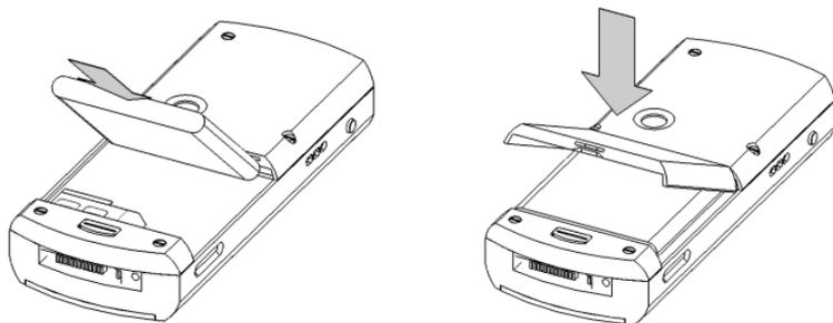
Slide the release button down and place the battery cover back in place.
